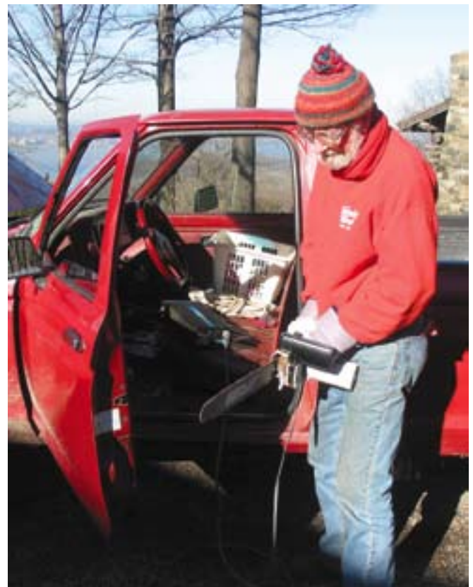
Pete's electric chain saw runs off of an inverter installed in the pickup.
